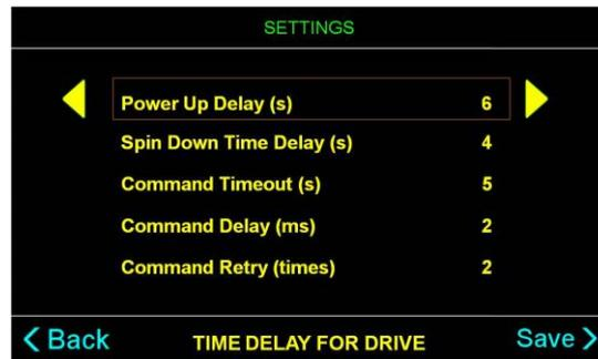
Figure 40: Set Time Delay for Drive
