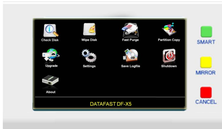
Figure 5: Front Panel with LCD, status LED and control buttons
