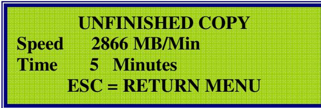
When you press **ESC** to turn back to the sub menu, the DF1 will automatically power off the drives, so that is safe for you to replace any drive if you want.
